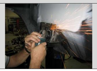
Prep the firewall mounting surface edge on the firewall side by grinding smooth the flange edge so that the TCI clip will be mounted flush to the firewall.
