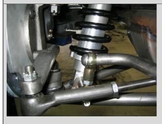
Complete installation by fastening the upper  $\frac{1}{2}$  inch rod end of the sway bar link from the lower shock mount bolt to the end of the anti-roll bar with the  $\frac{1}{2}$ -20 x 1  $\frac{1}{2}$  inch button head bolt.
