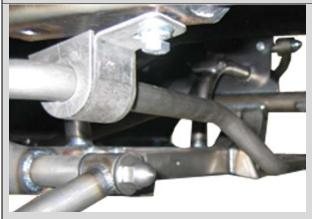
Install the front anti-roll bar into position using the supplied polyurethane and saddle mount making sure that the stepped down center section is down to clear the engine pulley. Fasten anti-roll bar saddle mount using the supplied  $3/8-16 \times 1$  inch hex head bolt; 3/8 inch lock and flat washer.
