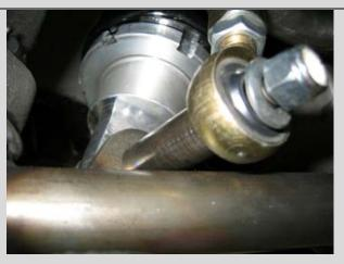
Next, install the shock into the lower a-arm tabs making sure that the adjustment dial towards the rear of the vehicle and install the  $3\,\%$  inch shoulder bolt from the rear through the rear bracket, then the shock bearing, front bracket, then the spacer and last the rod end link for the sway bar. Install the washer and nut and tighten. The top rod end will be attached to the sway bar later.
