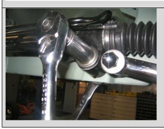
Install the rack & pinion assembly using the two 5/8" in. bolts, washers and lock nuts supplied. On power rack and pinions units the 5/8 thick spacer goes between the rack brackets on the cross member and the rack. Install the tie rod ends onto the rack and into the spindle steering arms.
