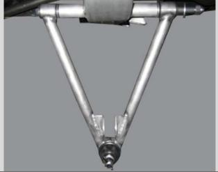
Continue with the front suspension component installation. First, install the lower control a-arm shaft with acorn nut towards the front of the car into lower A-arm (shock mounting tabs facing up) and though the cross-member, the washers go on each side of the bushings.
