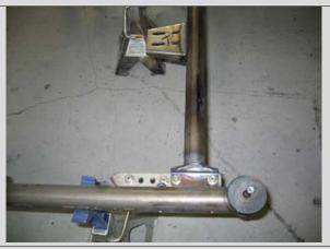
Mount the emergency brake cable bracket on the driver side with the same mounting point as the transmission cross-
